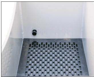
Shown is slatted flooring, and dryer hose attachment. Other attachment is on facing side and to the back to create circular air flow
